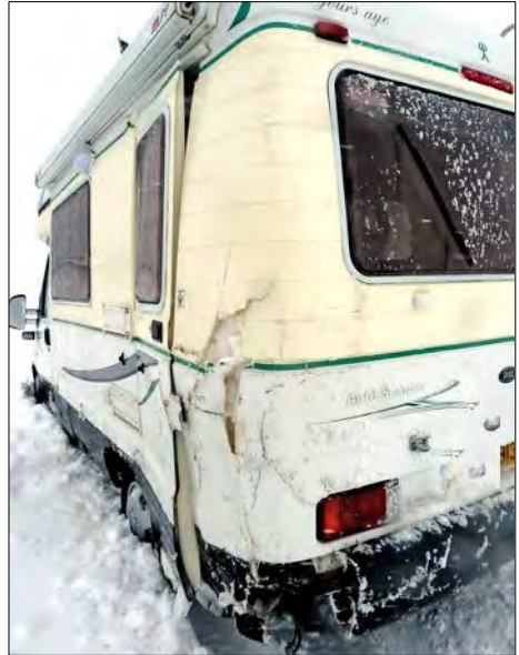
above: damage to motorhome after being hit by a 25 tonne coach
